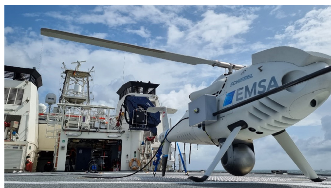
EMSA RPAS located on the helideck of the patrol vessel of the German Federal Police. The air vehicle is equipped with special gas sensors (grey box and pipe on the flank) and optical cameras (turret on the belly). (Photo credits: Schiebel)
