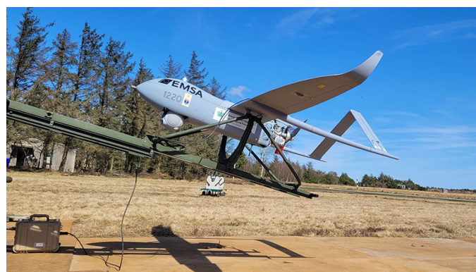
The Aerosonde RPAS uses a catapult for take-off and is recovered with a net. It has an endurance of ten hours and a radio range of 140 km. (Photo credits: EMSA)
