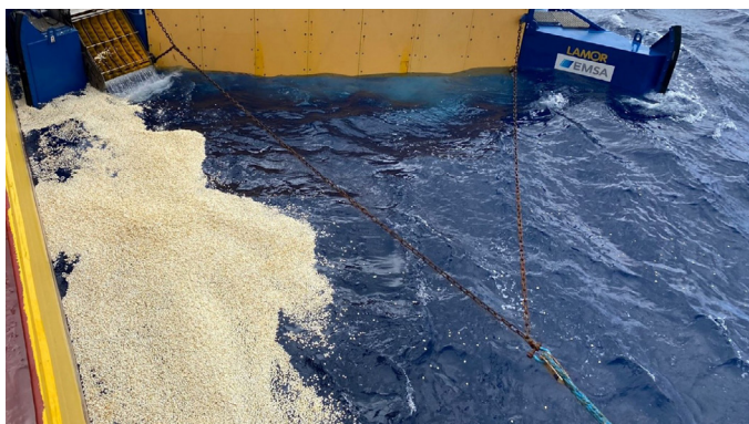
Demonstrating the ability to recover oil spills by collecting simulated spill material, in this case popcorn
